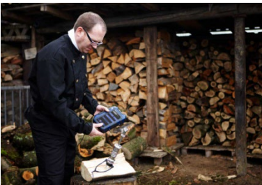
Fig. 40: Wood moisture measurement with Probe Wöhler HBF 420.
