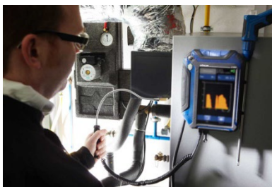
Fig. 45: Spillage test: Searching for condensate
