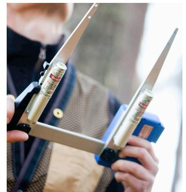
The image shows Gator Eyes laser pointers installed on the Digitech Professional caliper. When Gator Eyes are installed, the total weight of your caliper will increase with approx. 190g./7,6oz.
