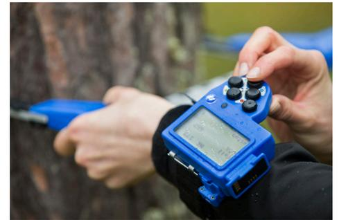
The DP II computer terminal placed on the wrist and with the SmartScale used to measure standing tree diameters. This work mode is possible by using the Radio Enter button (factory assembled) on the SmartScale to send data to the computer terminal for storing and processing.
