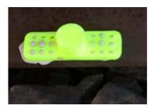
The base plate is made of a semi-porous polymer, which is light, easy to use and very durable. It's design includes eighteen holes which allows the adhesive to move through and over the base, greatly increasing adhesion. This prevents movement and avoids unnecessary re-fitting of targets.
