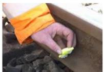
**Step Two** — The target or flag is attached to the base plate in one of the sets of slots appropriate for the angle from which readings will be taken.
