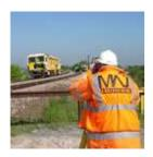
In the image to the left an engineer can be seen taking the same readings whilst the line is in use without inhibiting rail traffic. The target allows all track monitoring work to be undertaken in a position of safety with the minimum amount of disruption and far fewer staff involved in the process.
