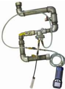
Fig. 55: Volume measurement with the Wöhler DC 410 FLOW and a syringe (up to 100 ml tube volume).
