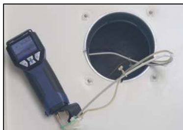
Fig. 31: Example - Connection of the measuring hoses
