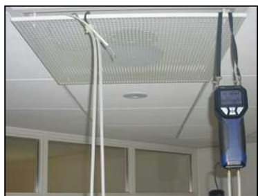
Fig. 33: Example - Fixing with the supporting loop
