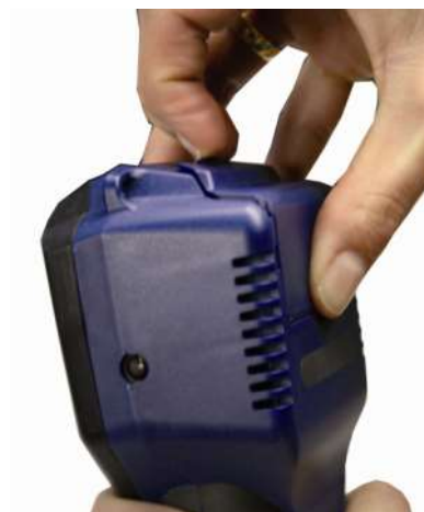
Fig. 10: Open the battery compartment.
