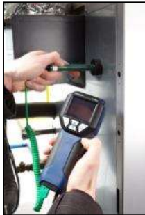
Fig. 53: Application example DC 430 Flow with Special Wall Temperature Probe
