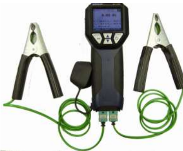
Fig. 4: Connecting a temperature measuring plier
